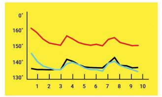
Each machine was run for ten minutes. They were run in 8 second cycles with 4 seconds of spray and 4 seconds of rest. Every three minutes there was a 15 second rest. The temperature was recorded at the tip on the end of a 20 foot solution hose. These charts show the true temperature maintained after the initial burst of heat.
